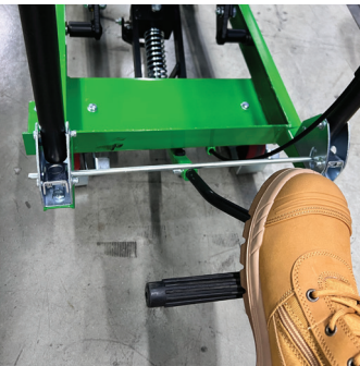
Foot lever activated by downward pressure for easy lift operation.
