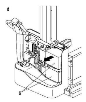
Installation is in the reverse order of operations, pay attention on battery install position and cable connection. Make sure the well place cables to avoid be damaged when you removal and installation battery.
